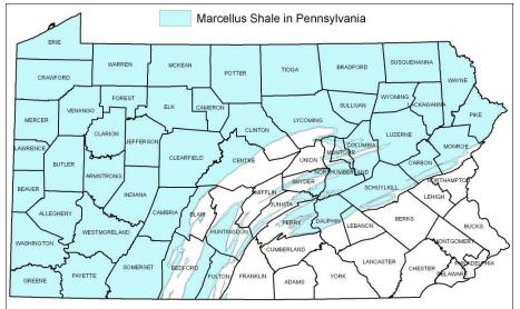
The Marcellus Shale formation contains a high grade of natural gas, and covers nearly the entire Appalachian region of Pennsylvania. The shale varies in depth from surface outcrops to more than 8,000 feet deep. Recent drilling techniques enable gas drillers to now reach the deeper parts, making widespread drilling economical.
